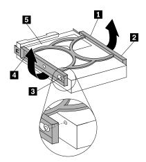
Figure 36. Installing the hard disk drive into the bracket
